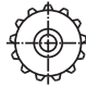
SAE-B Splined shaft Class 1-J498b 16/32 dp.13 teeth 30° PA flat root side fit.
